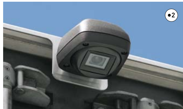
A better view: optimum visibility is ensured by the modified mirror array (1) with the upper wide-angle mirror on the driver's side and, below it, the main mirror, as well as by the optional reversing camera (2). The one-piece sunblind (3) offers effective dazzle protection even when the sun is low in the sky
