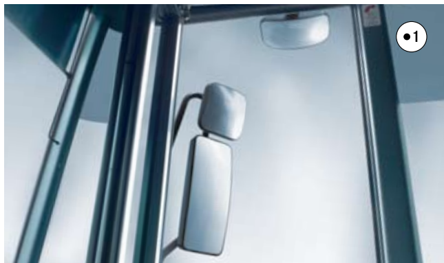
A better view: optimum visibility is ensured by the modified mirror array (1) with the upper wide-angle mirror on the driver's side and, below it, the main mirror, as well as by the optional reversing camera (2). The one-piece sunblind (3) offers effective dazzle protection even when the sun is low in the sky
